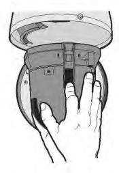
Figure 2. Dome Drive Installation
