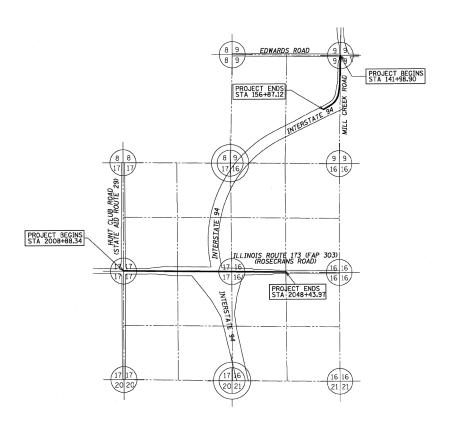
PROJECT LENGTH = 3955.63 LINEAL FEET (0.749 MILES), ILLINOIS ROUTE 173 1488.22 LINEAL FEET (0.282 MILES), MILL CREEK ROAD
