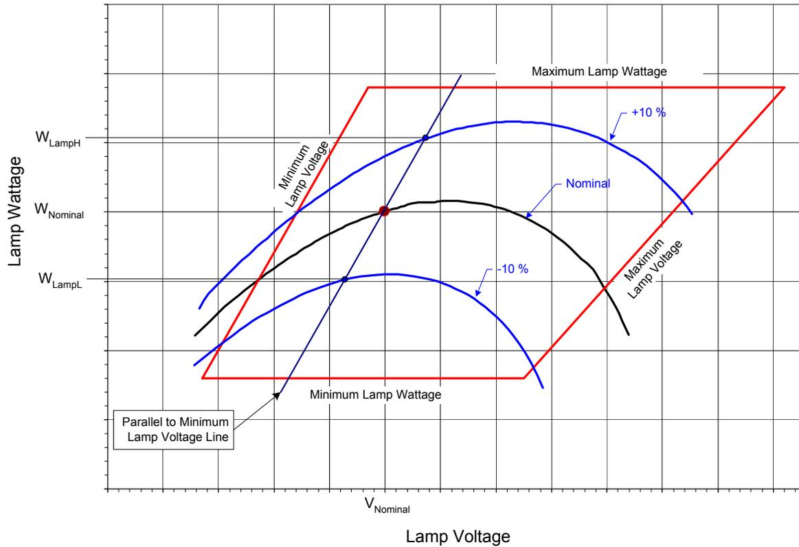
$$\text{Ballast Regulation} = \frac{W_{LampH} - W_{LampL}}{W_{LampN}} \times 100$$
