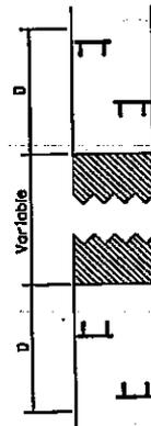
Type III Barricades and RI-4-4830 signs shall be set up as shown in 'Traffic' detail on Highway Standard 702001. If the distance 'D' exceeds 600 m (2000') an additional set of barricades and RI-4-4830 shall be placed at each end of the work area.
