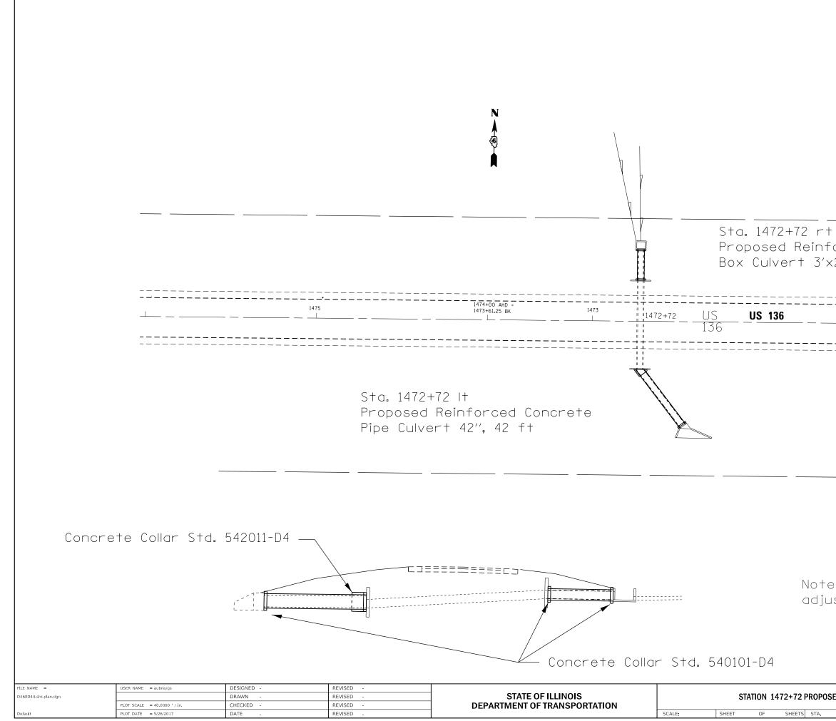
Proposed Reinforced Concrete Box Culvert 3'x2.5', 18 ft
