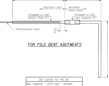
Min. Pull-out Strength = 9.2 kips - tension No. Required = N/A
