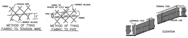
WHERE FENCE LINE HAS A CHANGE IN DIRECTION OF 15' OR MORE, A TERMINAL POST SHALL BE PLACED AS SHOWN ABOVE.
