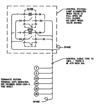
CONTROL STATION WIRING DIAGRAM (TYP. OF TWO)
