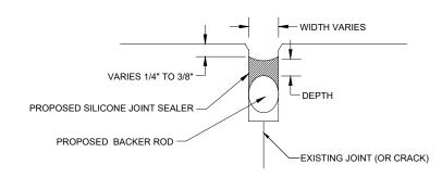
CONCRETE JOINT CLEANING AND SEALING DETAIL
