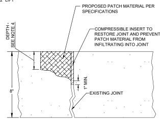
PARTIAL DEPTH SPALL REPAIR SECTION VIEW
