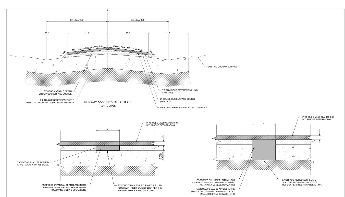
AR401915 REMOVE & REPLACE BITUMINOUS PAVEMENT - TYPE A (PARTIAL DEPTH)
