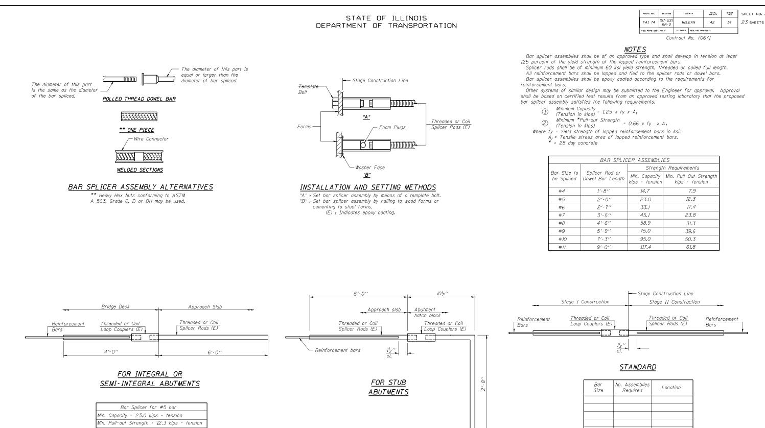
Bar Splicer for #5 bar Min. Capacity = 23.0 kips - tension
