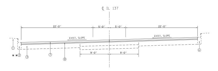
PROPOSED TYPICAL SECTION ILL (137) / BUCKLEY ROAD STA. 135+00 TO STA. 151+67 SUPERELEVATED CROSS SECTION
