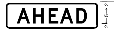
W16-9p_30x9 FLYG; 1.5" Radius, 0.5" Border, 0.4" Indent, Black on Bright yellow green; [AHEAD] D 2K 125% spacing;
