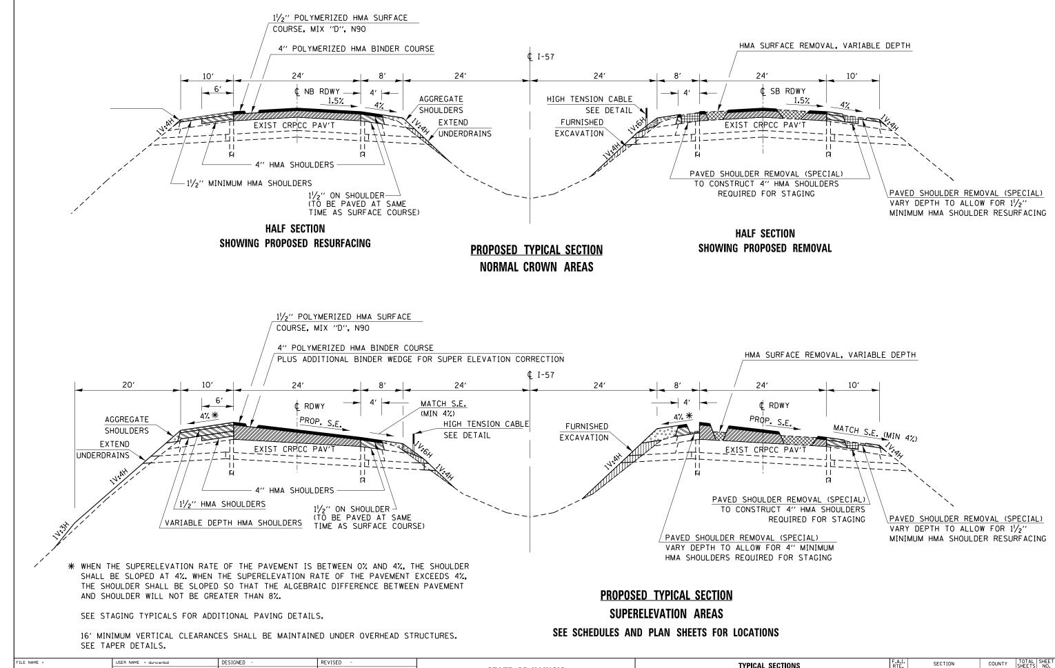
TYPICAL SECTIONS STATE OF ILLINOIS :\pw\_work\pwidot\duncanbd\d0315542\D36BC53-sht-tupical.don DRAWN REVISED (38-3)RS-2 IROQUOIS 186 10 PLOT SCALE = 100.0000 '/ in. CHECKED REVISED **DEPARTMENT OF TRANSPORTATION** CONTRACT NO. 66C53 SCALE: SHEET OF SHEETS STA. TO STA. PLOT DATE = 6/10/2014 DATE REVISED
