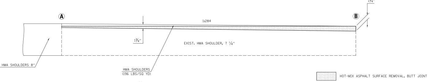
st - EXISTING PAVEMENT AT THIS LOCATION CONSISTS OF A TYPE B GUTTER BELOW THE  $7^1/4^{\prime\prime}$  HMA SHOULDER
