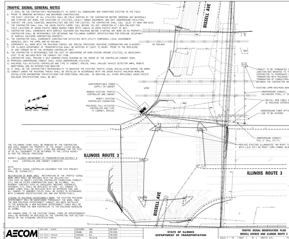
CONDUIT TO BE TERMINATED INTO THE BUNGALOW OR JUNCTION BOX MOUNTED TO THE BUNGALOW (IF PRESENT). CONTRACTOR TO COORDINATE EXACT CONDUIT TERMINATION WITH RAILROAD FORCES IN THE FIELD. TERMINATION OF CONDUCTORS/CABLE TO BE COORDINATED BETWEEN THE CONTRACTOR AND RAILROAD FORCES.
