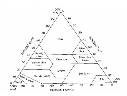
The mechanical analysis shall show that the % sand, % silt, and the % clay must yield a silt loam soil. See the attached Textural Classes diagram above. To determine the class plot a line parallel to the % clay axis starting the line at the value of the % silt. Plot another line parallel to the % sand axis starting the line at the value of the % clay. The intersection of these lines shall be in the silt loam region, for the soil to be approved.
