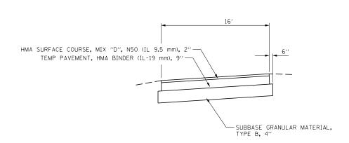
HMA SURFACE COURSE, MIX "D", N50 AND HMA BINDER (IL-19) mm ARE PAID FOR AS "TEMPORARY PAVEMENT".
