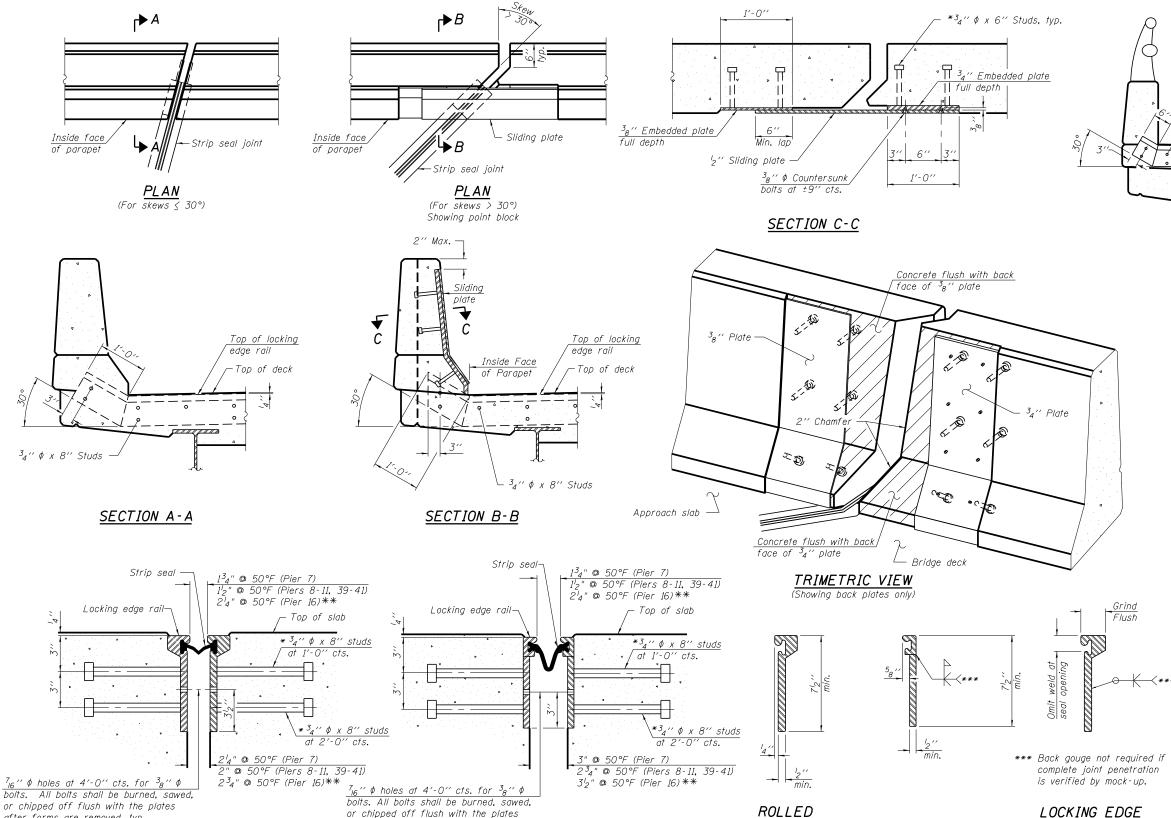
SECTION THRU ROLLED RAIL JOINT
