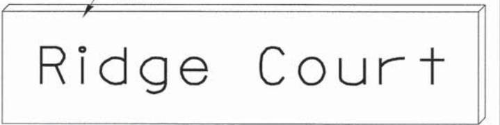
LED ILLUMINATED SIGN PANEL 8'0" x 2'6" (750 mm x 2.5 mm)(MAX.) C or D FONT
