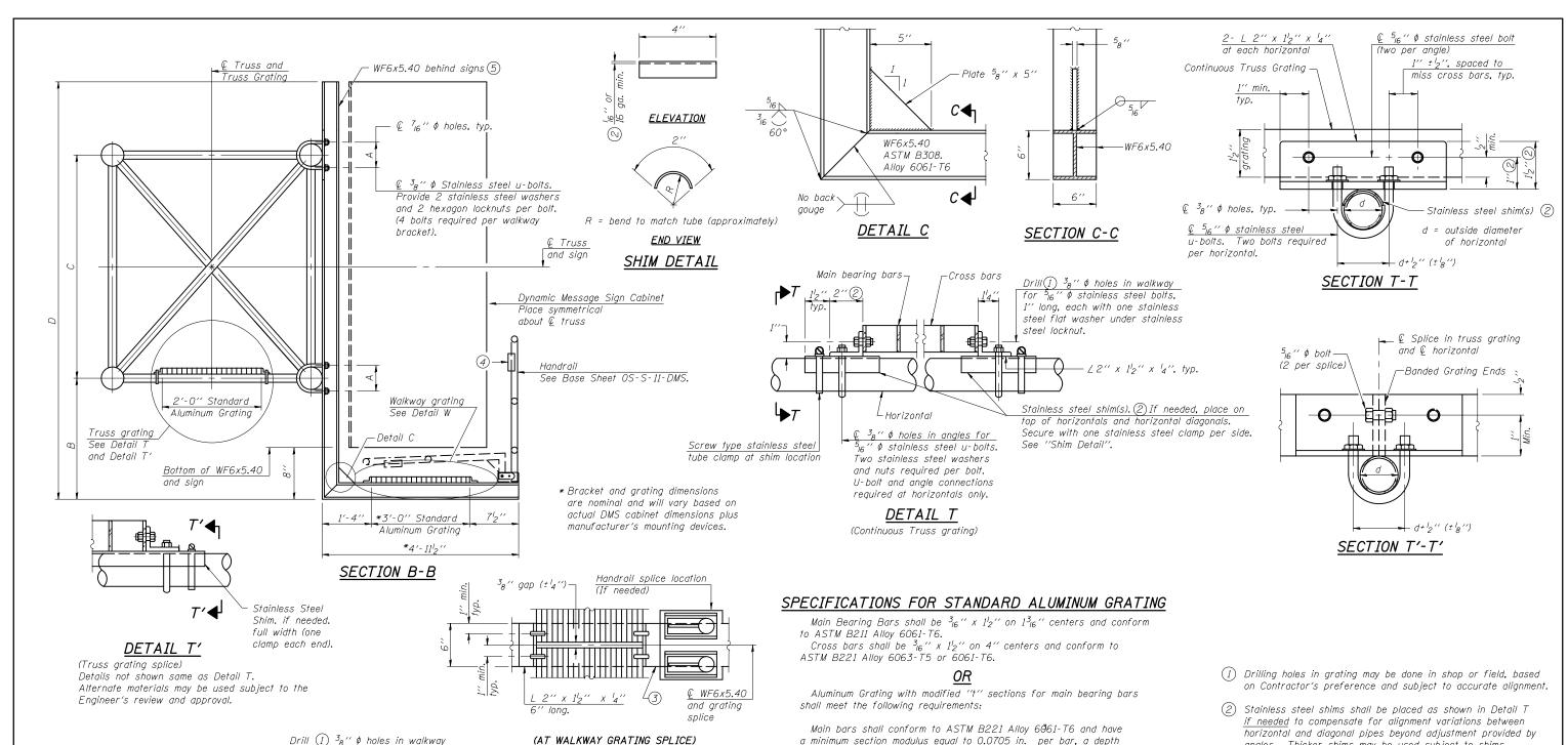
a minimum section modulus equal to 0.0705 in. per bar, a depth of  $I_2^{\prime\prime}$ , spaced on  $I_{16}^{3}$  centers. Cross bars shall conform to ASTM B221 Alloy 6063-T5 or T-42
