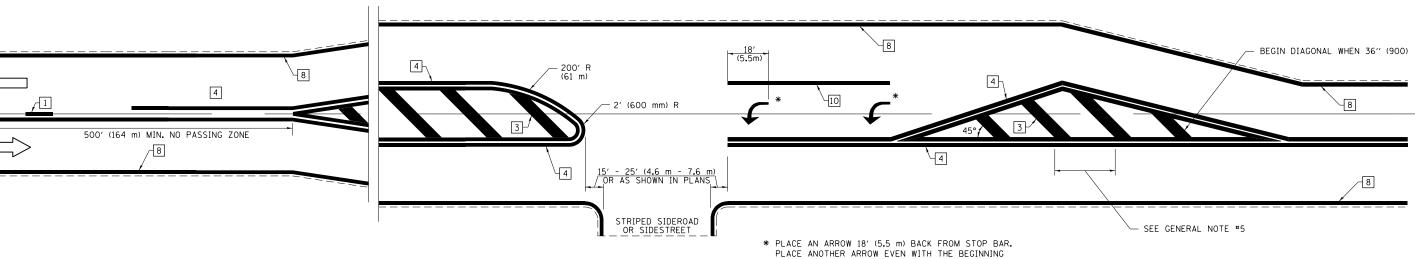
\* PLACE AN ARROW 18' (5.5 m) BACK FROM STOP BAR. PLACE ANOTHER ARROW EVEN WITH THE BEGINNING OF THE SOLID WHITE LINE. SPACE ADDITIONAL ARROWS EVENLY UP TO 80' (24.4 m) MAXIMUM SPACING. USE MINIMUM OF 2 ARROWS.
