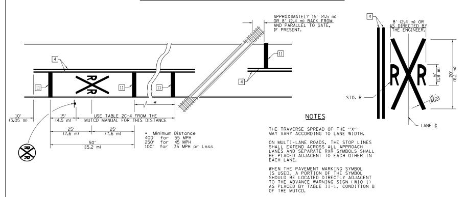
SUPPLEMENTAL PAVEMENT MARKING TREATMENT FOR RAILROAD-HIGHWAY GRADE CROSSING
