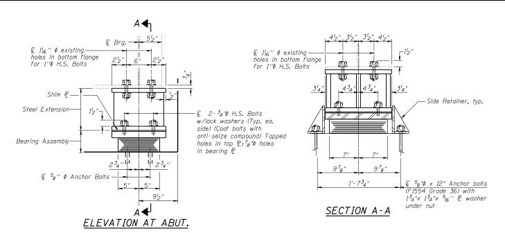
—Burn existing anchor bolts flush with existing concrete surface. Grind existing anchor bolt smooth and seal with epoxy. Cost is included with "Jack and Remove Existing Bearings".
