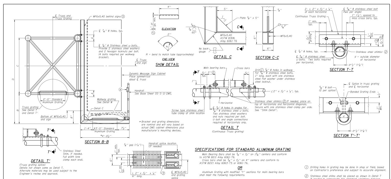
Main bars shall conform to ASTM B221 Alloy 6 $\ref{6}61$ -T6 and have a minimum section modulus equal to 0.0705 in. per bar, a depth of  $1'_2$ ", spaced on  $1^3_16$ " centers.
