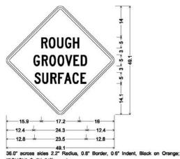
36.0" across sides 2.2" Radius, 0.8" Border, 0.6" Indent, Black on Oran [ROUGH] C 2K 81% spacing; [GROOVED] C 2K 91% spacing; [SURFACE] C 2K 85% spacing;
