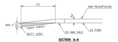
\*MILLING DEPTH SHALL BE A MAX OF 1 1/2" WHEN SIDEROAD OR ENTRANCE IS CONCRETE.
