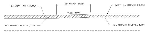
NOTE: THE TRANSITION FROM 2.25" TO 1.5" WILL BE INCLUDED IN THE PAY ITEM PROPOSED HMA SURFACE REMOVAL, 2.25".
