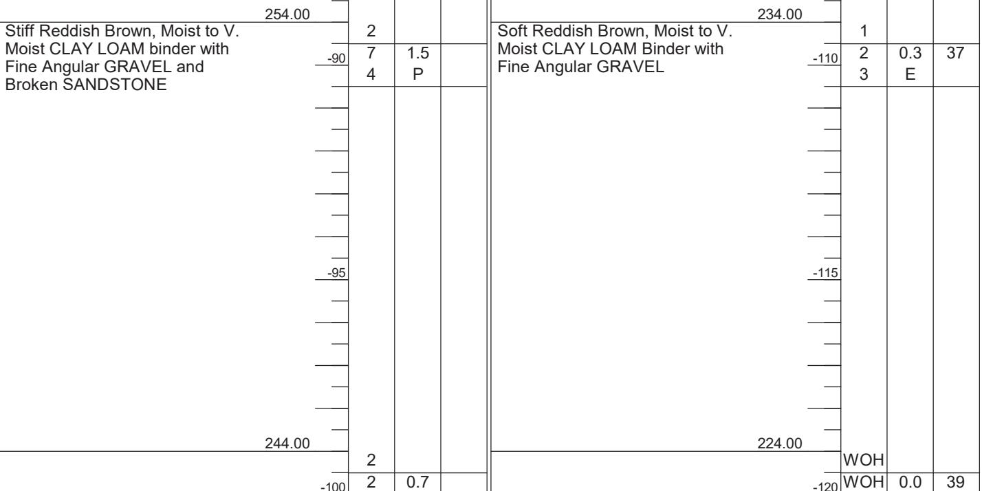
The Unconfined Compressive Strength (UCS) Failure Mode is indicated by (B-Bulge, S-Shear, P-Penetrometer, E-Estimated)
