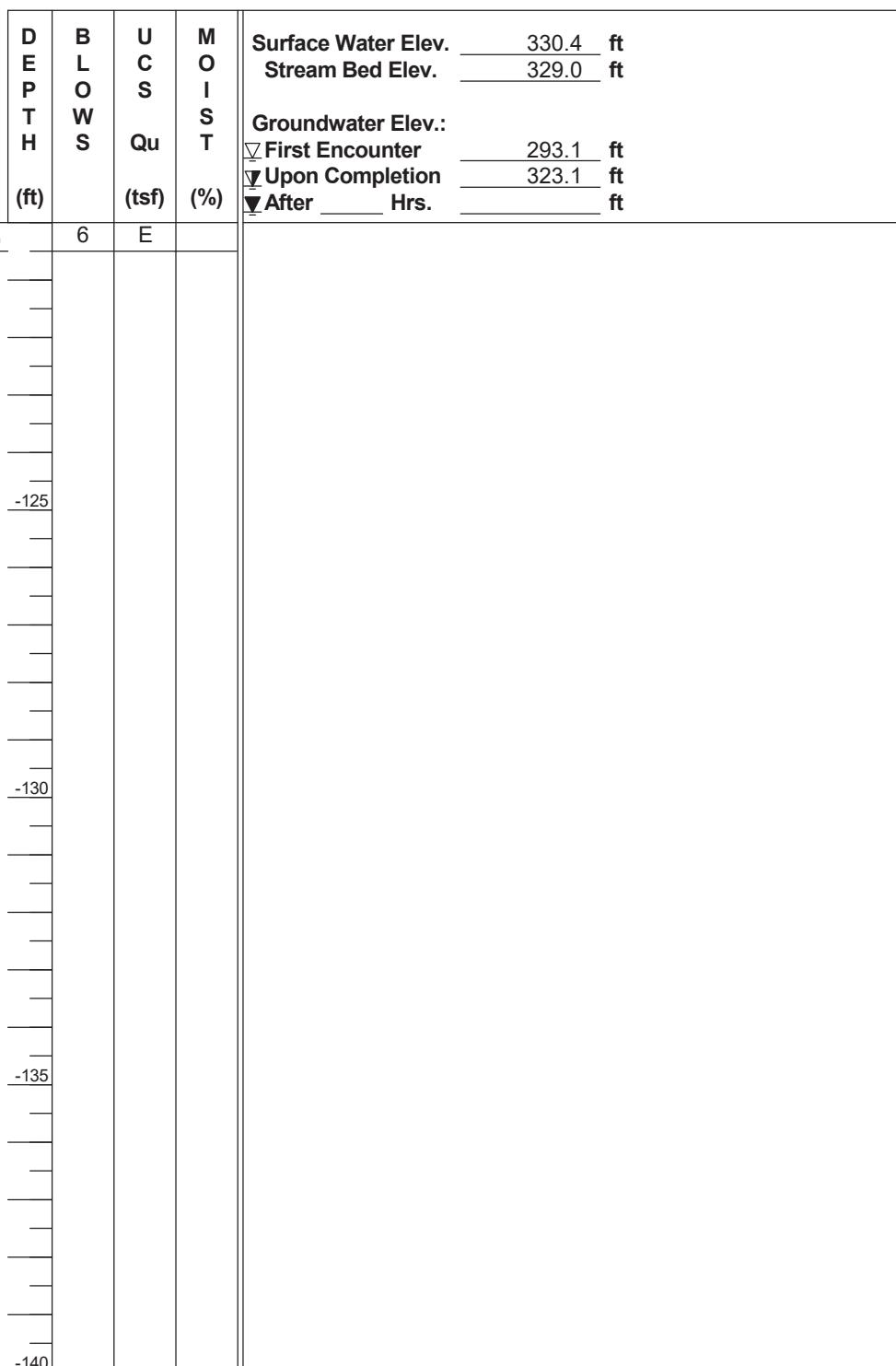
The Unconfined Compressive Strength (UCS) Failure Mode is indicated by (B-Bulge, S-Shear, P-Penetrometer, E-Estimated)
