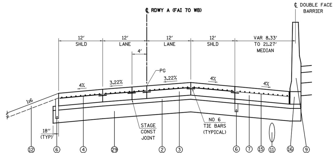
**PROPOSED ROADWAY A SUPERELEVATED SECTION**
