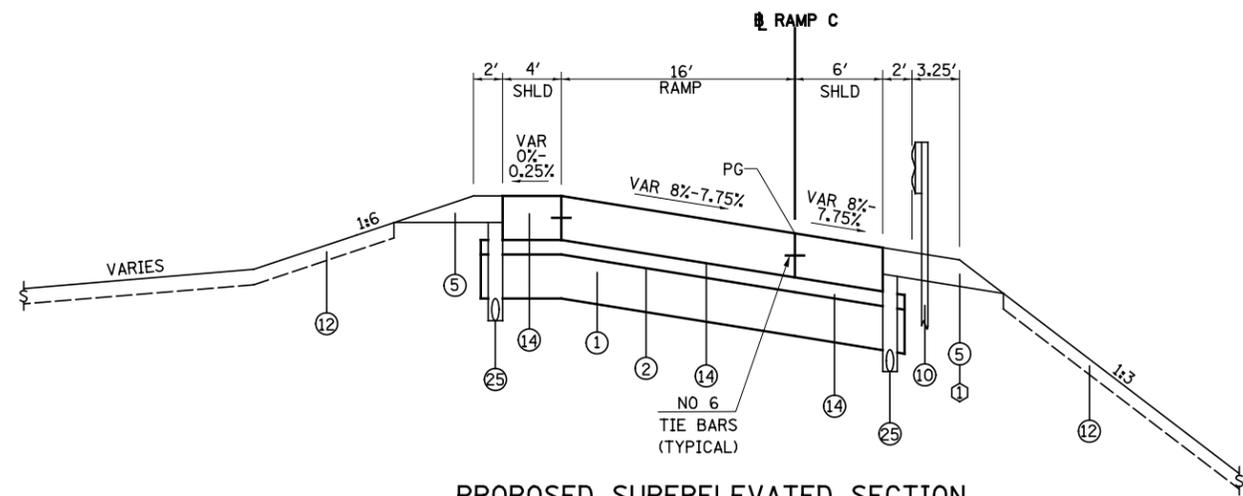
**PROPOSED SUPERELEVATED SECTION**
