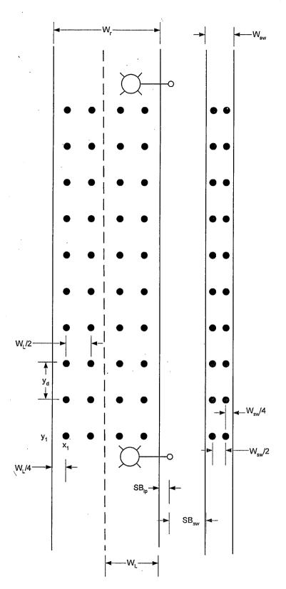
$W_r$  = Roadway Width  $W_L$  = Lane Width  $W_{SW}$  = Sidewalk Width  $SB_{LP}$  = Light Pole Set Back  $SB_{SW}$  = Sidewalk Set Back
