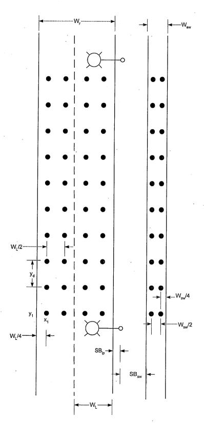
$W_r$  = Roadway Width  $W_L$  = Lane Width  $W_{SW}$  = Sidewalk Width  $SB_{LP}$  = Light Pole Set Back  $SB_{SW}$  = Sidewalk Set Back
