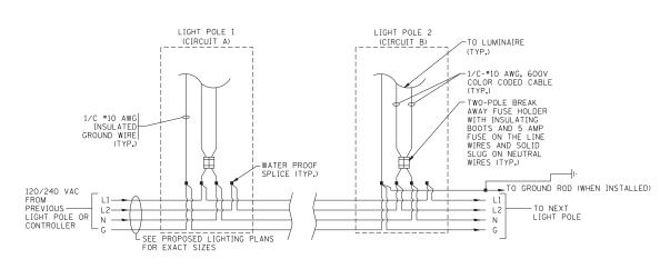
LIGHT POLE WIRING DETAIL NOT TO SCALE
