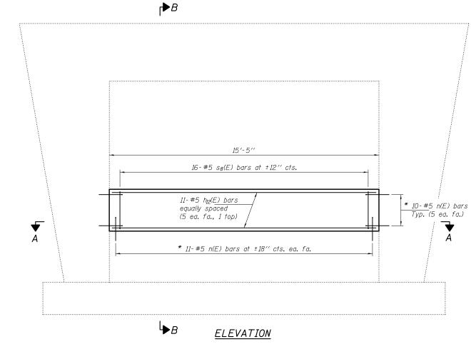
\* Epoxy grout n(E) bars in 9" min. holes according to Article 584 of the Standard Specifications.
