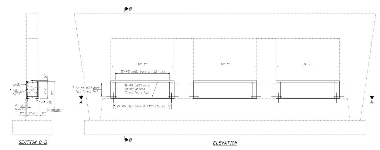
\* Epoxy grout n(E) bars in 9" min. holes according to Article 584 of the Standard Specifications.
