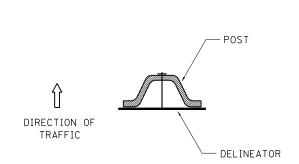
DELINEATORS SHALL BE INSTALLED ACCORDING TO STANDARD 635001 EXCEPT THAT THE POST SHALL BE ROTATED 180°. THE POST WILL HAVE THE WIDE SIDE FACING TRAFFIC AND THE DELINEATOR ATTACHECD AS SHOWN ABOVE.
