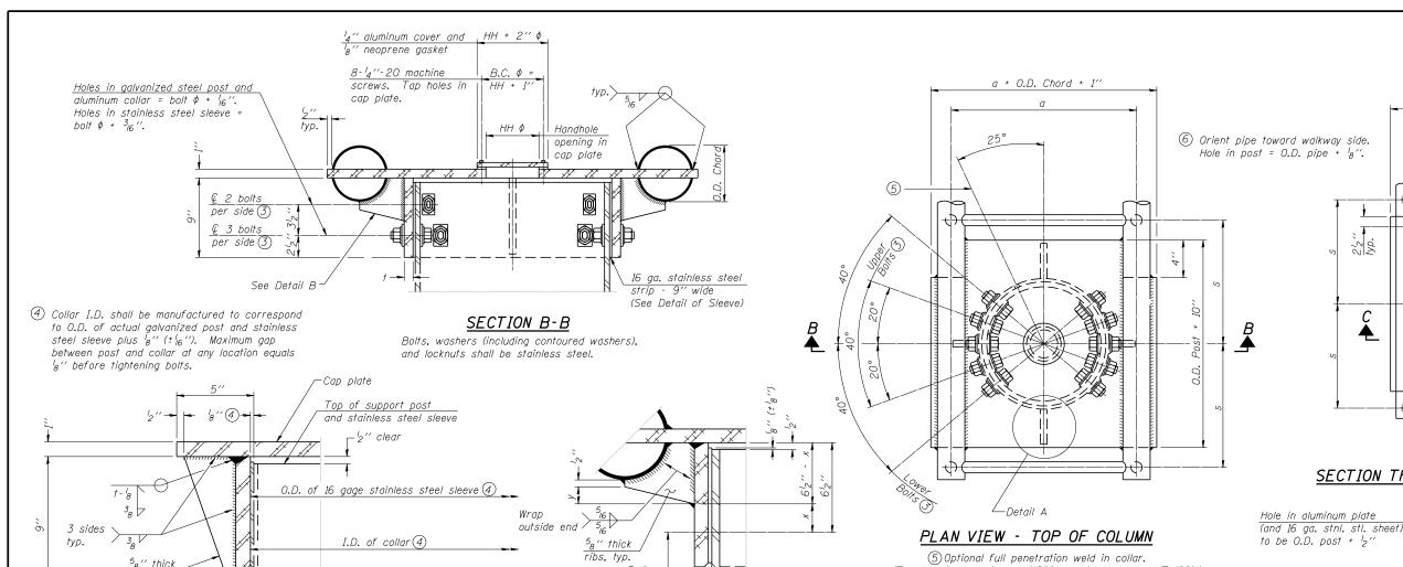
(5) Optional full penetration weld in collar. (Two locations maximum....(180° apart)....X-ray or UT 100%)
