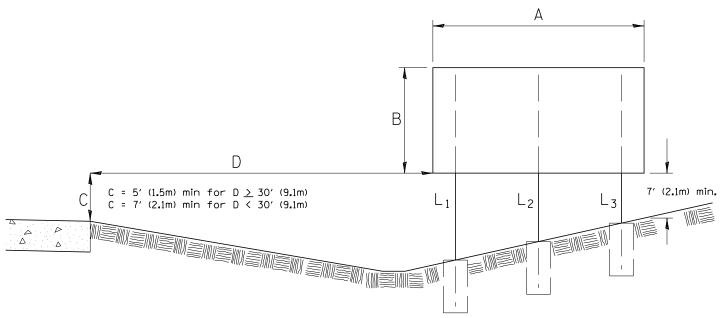
L<sub>1</sub> is always the post nearest to the edge of pavement. (See Sign Structures Manual)
