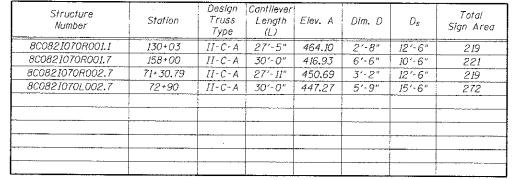
Alternate Vertical Diagonal Bracing for Each Sign Panel Bay in Planes of Front and Back Chords Walkway, railing and lights (if required) omitted for clarity Cantilever Length (L) and Basis of Payment Post Support (along € of truss) Elev. A Edge of (Location varies) Pavement THE THE THE THE TABLE A TANKAN Elev. A = Elevation at point of minimum clearance to sign, walkway support or truss.
