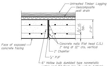
water seal (6" from top of wall to bottom) Cost included with Concrete Structures
