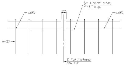
GFRP REBAR STIFFENING DETAIL
