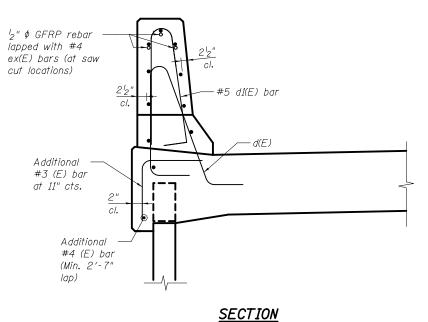
(Showing reinforcement clearances for slip forming and additional reinforcement)
