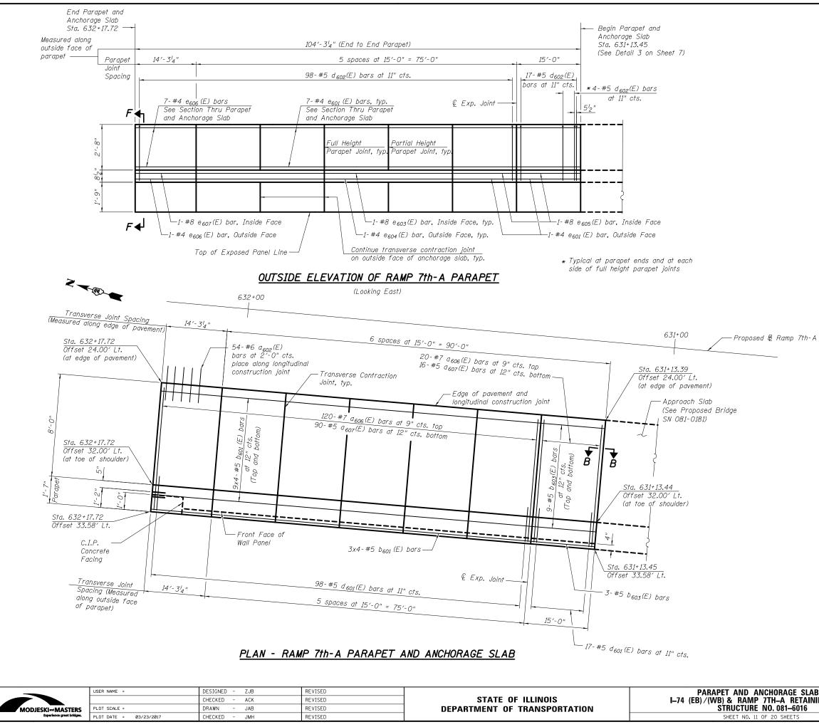
Joints in the adjacent pavement shall be aligned with the anchorage slab joints. Stations and offsets on this sheet are given to the
