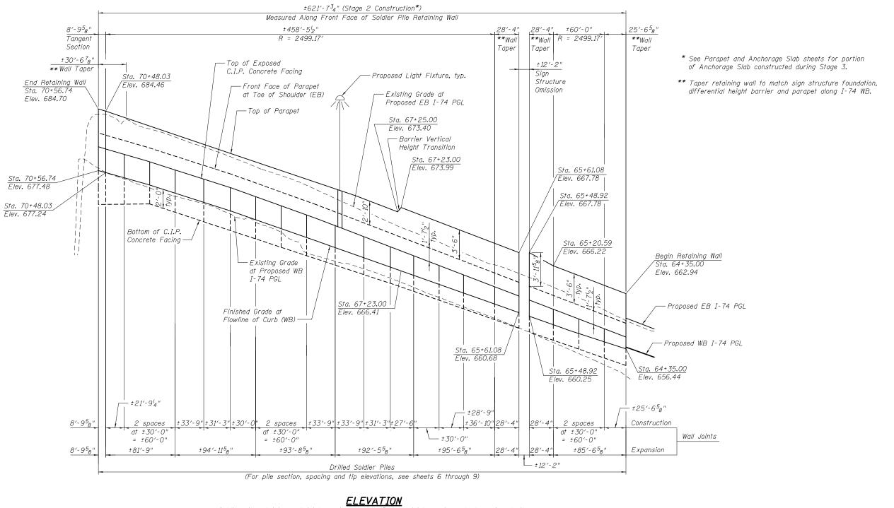
Soldier pile retaining wall joint spacing shown. Parapet joint spacing not shown for clarity.
