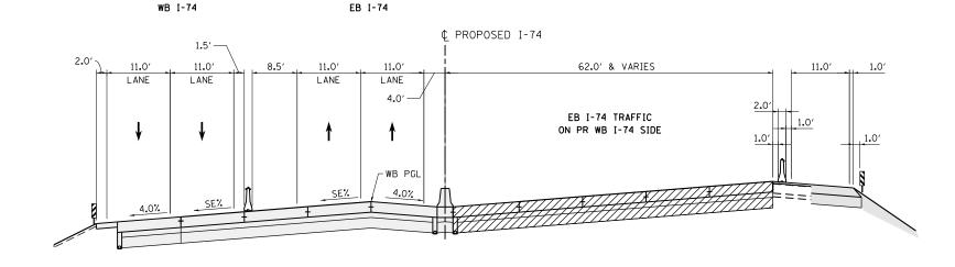
STAGE 3-1 I-74 MAINLINE TYPICAL SECTION PR I-74 STA 117+35.00 TO STA 122+00.00
