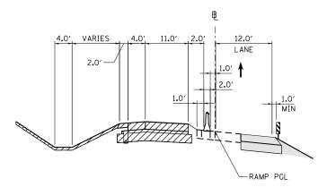
STAGE 3-1 AVENUE OF THE CITIES RAMP RAC-B TYPICAL SECTION PR RAMP RAC-B STA 924+83.48 TO STA 928+51.77
