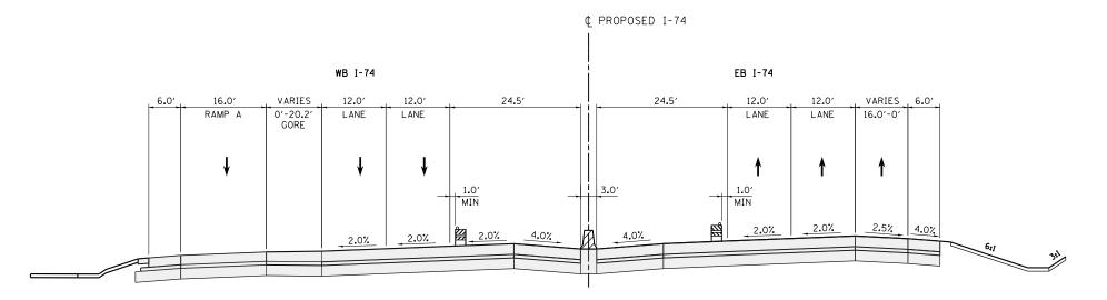
STAGE 3-4 I-74 MAINLINE TYPICAL SECTION PR I-74 STA 122+00.00T0 STA 129+75.00
