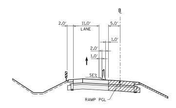
STAGE 3-2 AVENUE OF THE CITIES RAMP RAC-B TYPICAL SECTION PR RAMP RAC-B STA 924+83.48 TO STA 928+51.77
