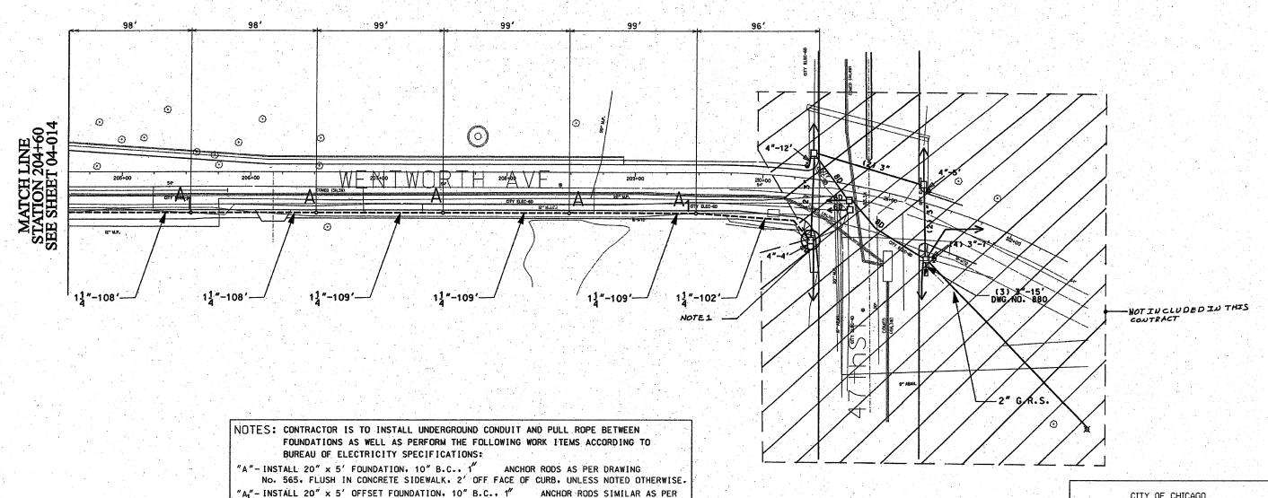
1 $\frac{1}{4}$ " DIRECT BORED CONDUIT SCHEDULE #80 AS PER IDOT ARTICLE 810.03 CONCRETE FOUNDATION - 5'  $\times$  20". 10" B.C.. 1" ANCHOR RODS OFFSET CONCRETE FOUNDATION - 5'  $\times$  20". 10" B.C.. 1" ANCHOR RODS
