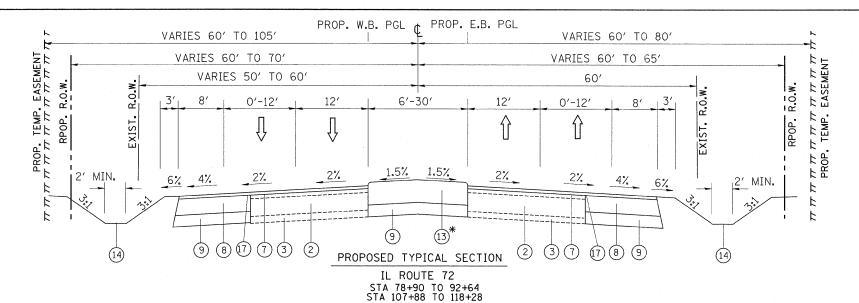
\*SEE THE ROADWAY PLAN SHEETS FOR THE LOCATIONS OF PROP. CORRUGATED MEDIAN NOTE: FROM STA. 78+90 TO 91+39 AND STA. 109+14 TO 118+278 PROP. PGL IS EXIST. ROADWAY CENTER LINE
