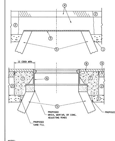
EXISTING BROKEN FRAMES AND LIDS SHALL BE REMOVED AND DISPOSED OF BY THE CONTRACTOR AND SHALL BE REPLACED AS DIRECTED BY THE ENGINEER. REPLACEMENT FRAMES AND LIDS WILL BE PAID FOR IN ACCORDANCE WITH ARTICLE 109.04 OF THE STANDARD SPECIFICATIONS UNLESS A SEPARATE PAY ITEM HAS BEEN PROVIDED.
