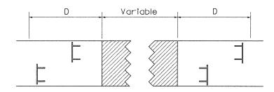
Type III Barricades and R11-4-4830 signs shall be as shown in "Road Closed To All Thru Traffic" detail on Highway Standard 701901. If the distance "D" exceeds 600 m (2000") an additional set of barricades and R11-4-4830 shall be placed at each end of the work area.
