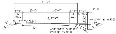
SUGGESTED FILL SECTION CONSTRUCT AS SHOWN BY STATION CROSS SECTIONS SUGGESTED CUT SECTION CONSTRUCT AS SHOWN BY STATION CROSS SECTIONS
