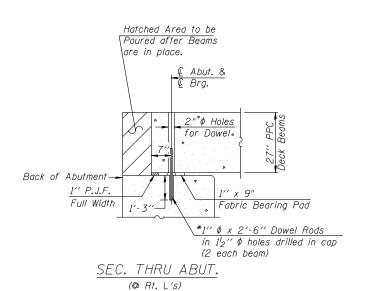
\* Note: After beams are in place,  $1_2^{\prime}$ " holes shall be drilled into the Substructure, and the dowel rods grouted in place and allowed to cure (Min. 24 Hrs.) prior to grouting shear key.
