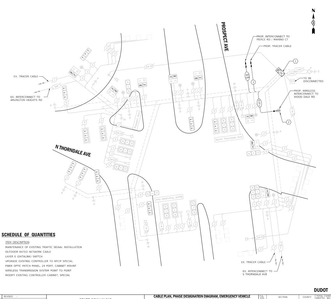
THIS INTERSECTION SHALL BE ADDED TO THE DUDOT CENTRAL SIGNAL SYSTEM AND REMOVED FROM THE EXISTING MULTIMODE NETWORK (ECON 111).
