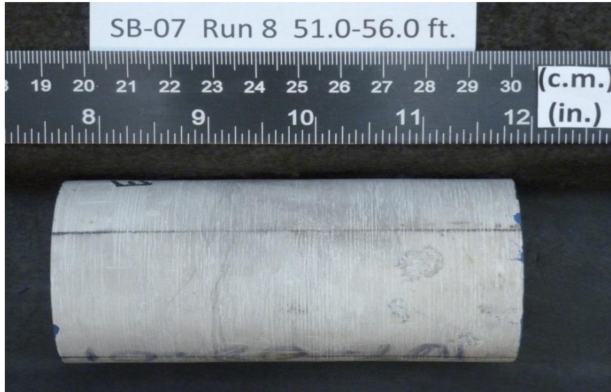
After cutting and grinding
