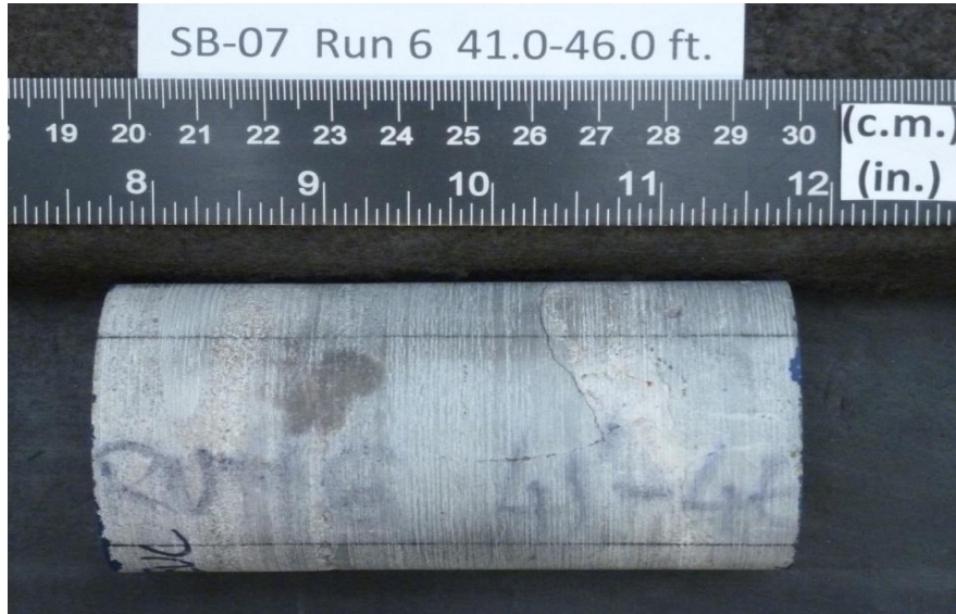
After cutting and grinding
