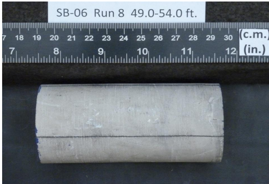
After cutting and grinding
