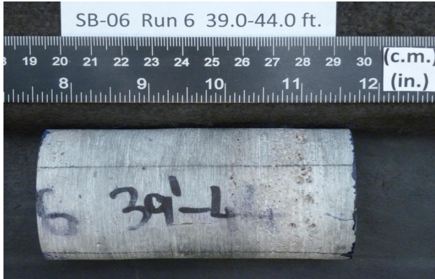
After cutting and grinding
