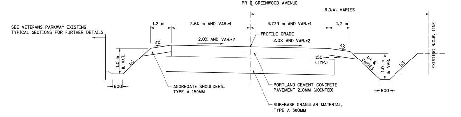
\*1 VARIES FROM 3.66 m LT & 4.733 m RT AT STA. 6+989.437 TO 4.5 m AT STA. 7+024.475 \*2 2.0% FROM STA. 6+989.437 TO STA. 7+010.000
