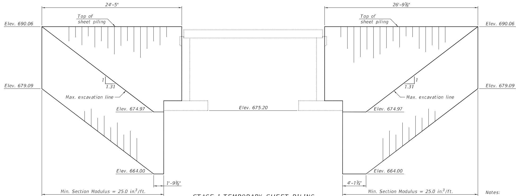
STAGE I TEMPORARY SHEET PILING (Looking West)
