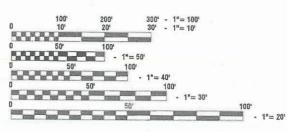
FULL SIZE PLANS HAVE BEEN PREPARED USING STANDARD ENGINEERING SCALES, REDUCED SIZED PLANS WILL NOT CONFORM TO STANDARD SCALES, IN MAKING MEASUREMENTS ON REDUCED PLANS, THE ABOVE SCALES MAY BE USED.
